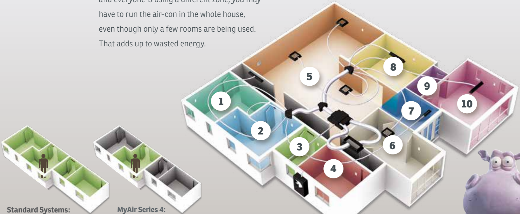
Standard Systems: If all bedrooms are on one zone, all rooms must be air-conditioned, even when some are not in use.
