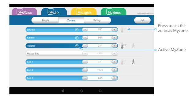
This feature can be particularly important when you have an unusually high requirement for air conditioning in a particular area. For example, a group of people watching a movie in Theatre room with all the electronic A/V equipment turned on will have a larger requirement for air conditioning than in other rooms in the house. Setting the Theatre as MyZone will ensure that the system continues running until the temperature set-point for that room is achieved.
