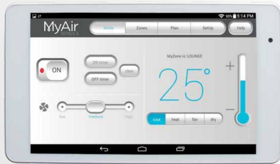
*The home screen gives you an overview of the air-conditioning status. Adjust the central temperature from this screen, or tap through to zones to fine-tune the airflow to every room.*
